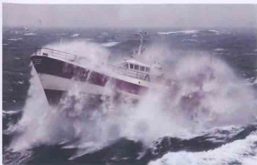
Plate 1 Hazardous sea conditions: the French fishing vessel Alf in storm conditions in the Irish Sea. As waves are tending to become higher, so are the dangers of foundering and capsizing during manoeuvres with fishing gear in bad weather.
