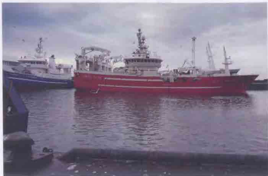
Plate 8 A very large pelagic vessel with advanced fish-finding and catching equipment capable of netting several hundred tonnes at every haul. The nets are pulled alongside and the fish pumped on board to cold tanks.
